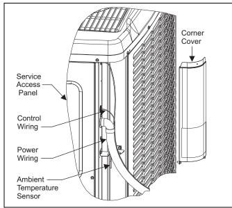
FIGURE 5: Typical Field Wiring
